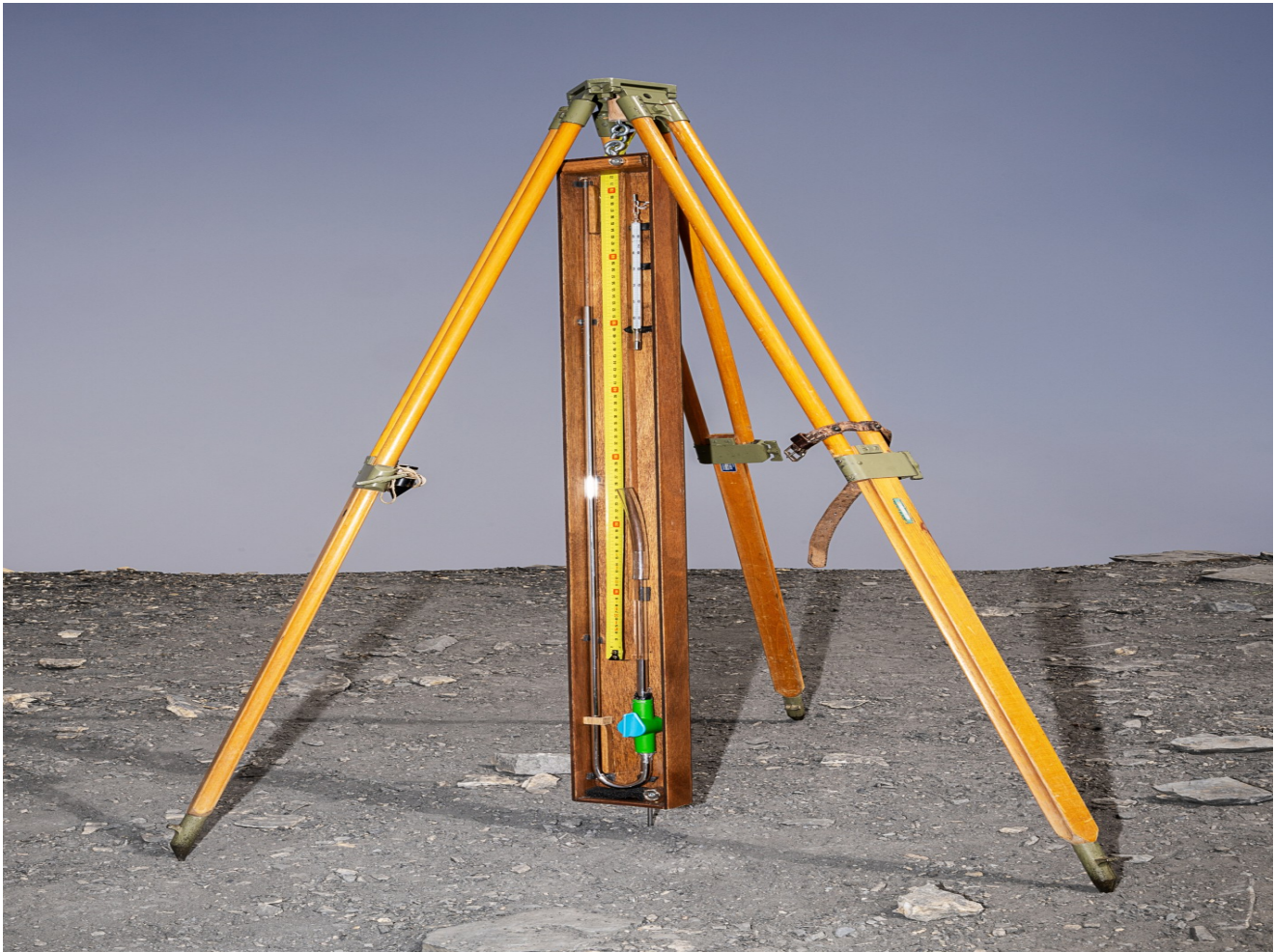
Figure 3. Contemporary replica of Deluc's barometer on the summit of Mont Buet (Assembled by Stéphane Fischer; Photograph © Olga Cafiero).
