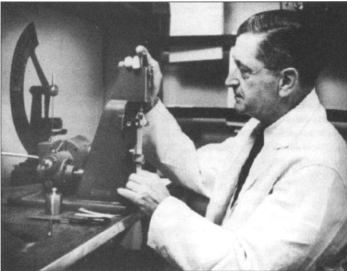
Figure 14. William J. Barrow in his laboratory conducting tests on the folding endurance of paper, from the Council on Library Resources' Fourth Annual Report, 1960. [Church 2005]
